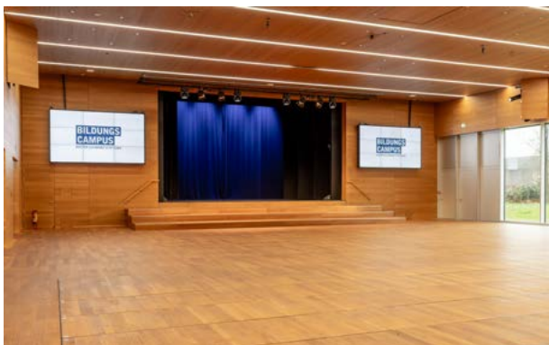
Tiered Forestage: The forestage can be moved backwards and forwards gradually, or you may select a larger stage surface. The display walls to the left and right may also be moved into different positions.
